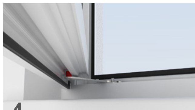
2 Insert the blockade base into the window frame about 60 mm from the inside edge of the window frame.
